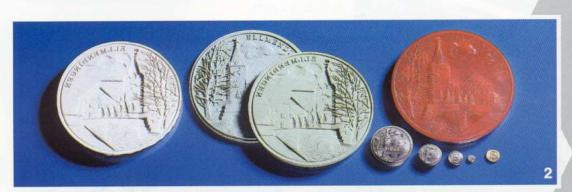
2 Working process: plaster model, silicone casting, scanning model, various work piece dimension
